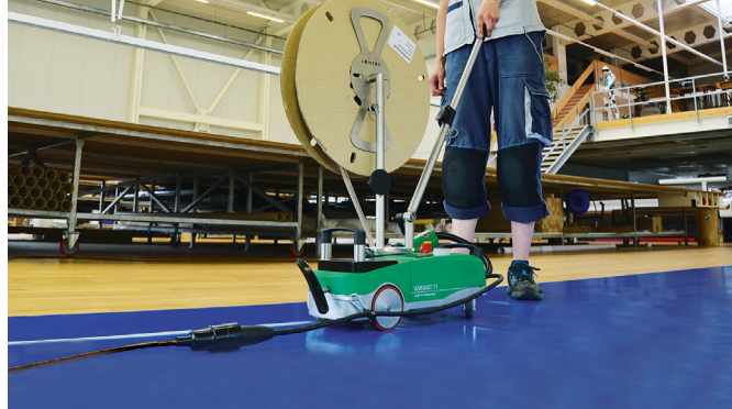
VARIANT T1 - wzmacnianie plandeki pasem PVC
