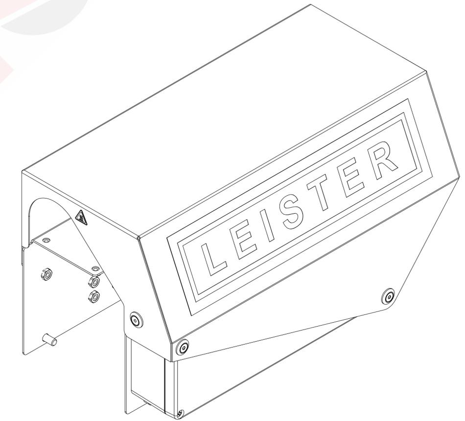
All screws secured with Loctite 242, 100.164
