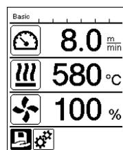
During operation, the setpoints of the welding parameters (drive in m/min or ft/min, temperature in degrees Celsius or Fahrenheit, air volume in percent and, if applicable, information notes are displayed (see Application Mode: Displaying current values).
