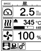
The air temperature actual value is lower than the setpoint.
