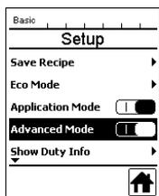
In the Basic setting, move through the Setup menu to save the recipe, to the Standby function ("Eco Mode") and Advanced Mode.
