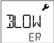
When the maintenance interval for the device is reached, the start display will show "BLOWER" or "DRIVE". The display disappears automatically after 10 sec. or can be acknowledged by pressing **Confirm key (42)**. You must take the device to your service center.
