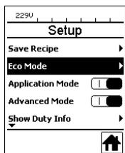
If the motor is switched off, the heating is activated, and if no key is pressed during the time defined under "Eco Mode" interval, then the device will switch over automatically to the Standby display. If the **"e-Drive" (31)** is not pressed during the subsequent 180 seconds, then the heating will switch to Cool Down mode. Standby will then appear on the display. Pressing **"e-Drive" (31)** causes the device to switch to Working mode.
